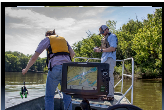
Side-scan sonar survey with Humminbird® fish-finder unit
