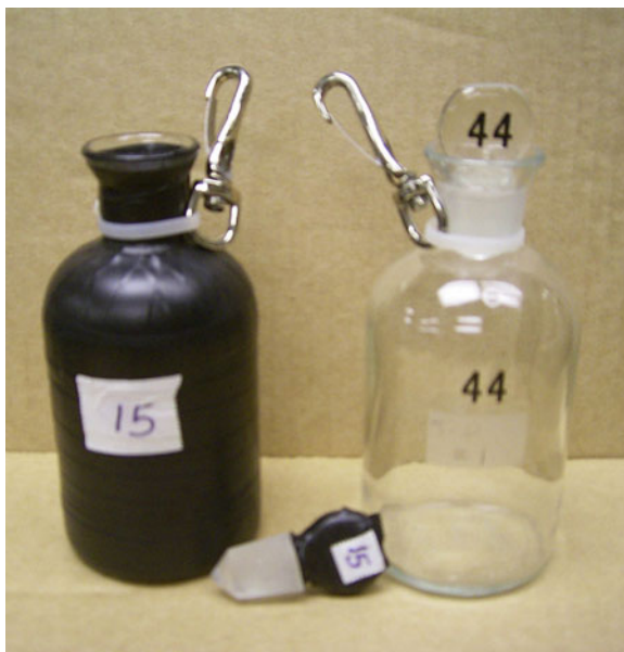
Fig. 1.8 Light and dark bottles for photosynthesis measurements
