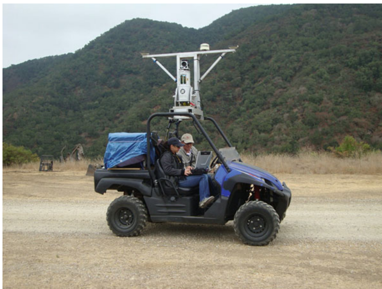
Fig. 2.14 An example of mobile terrestrial LiDAR positioned by RTK GPS and an inertial motion sensor that was used to map large tidal wetlands in central California
