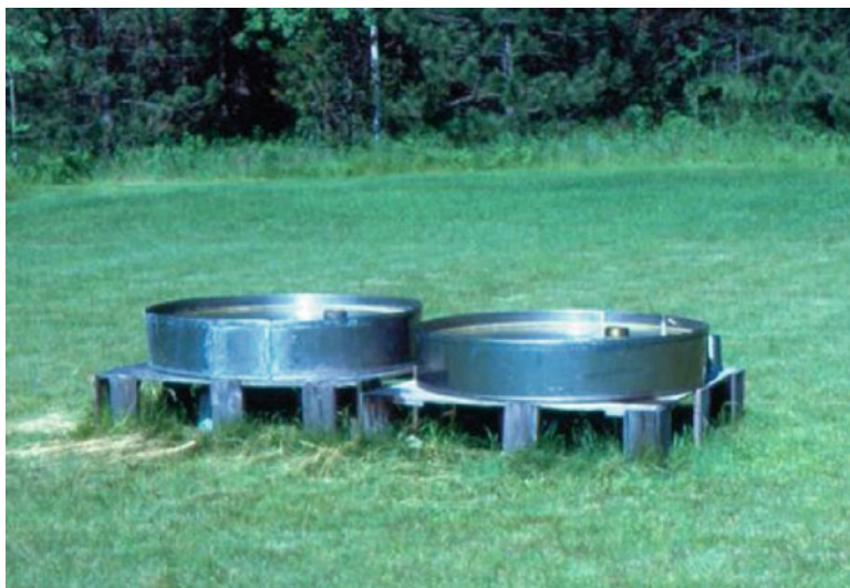
Fig. 3.8 Two standard class-A evaporation pans in use near a lake in northern Minnesota. One is serviced daily and the other weekly (Photo by Donald Rosenberry)
