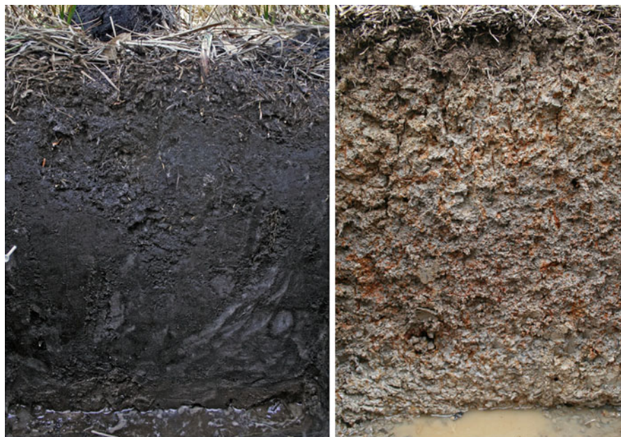
Fig. 4.13 Two hydric soils. The soil on the left meets Field Indicator S7 Dark Surface. The soil on the right meets Field Indicator F3 Depleted Matrix (Published with kind permission of US Department of Agriculture, Natural Resources Conservation Service (2010a). Figure is public domain in the USA. All Rights Reserved)
