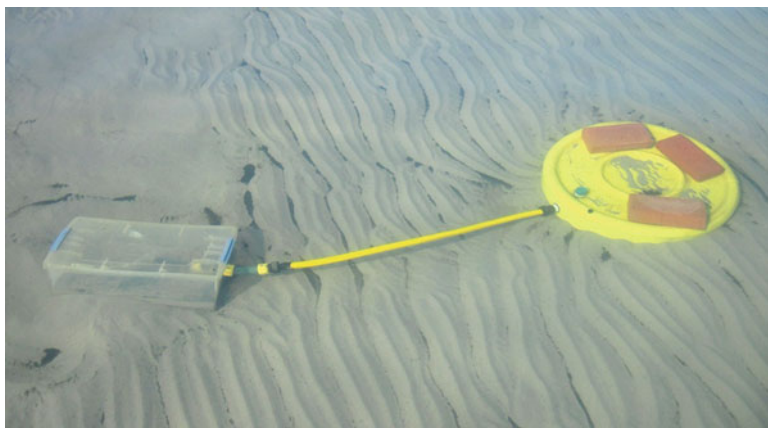
Fig. 3.45 Half-barrel seepage meter installed in sandy sediment. Note side port, to which the hose is connected, and top port with cap and vent hole with rubber stopper
