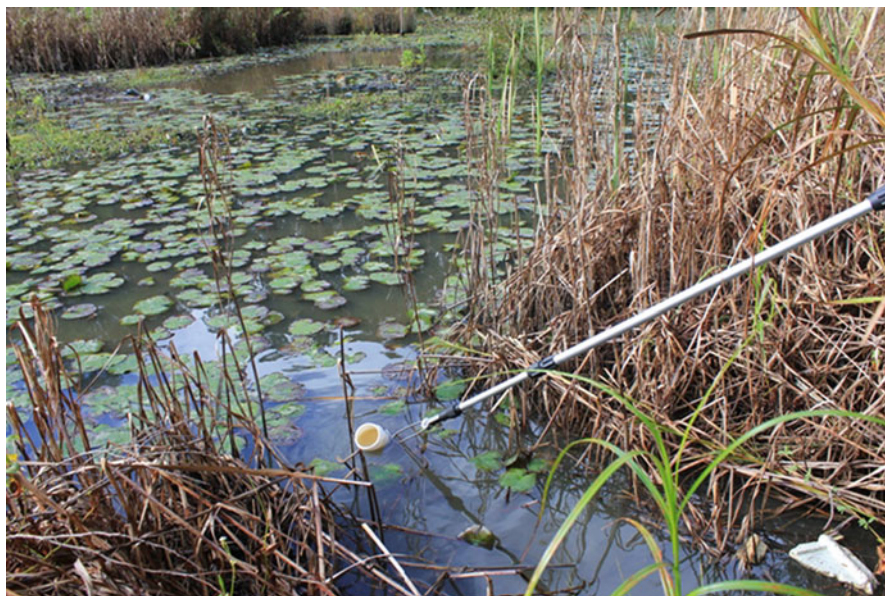
Fig. 6.2 A long-handled sampling pole with a collection bottle on the end can be used to avoid disturbing sediments and/or facilitate collecting water samples from deeper areas of the wetland
