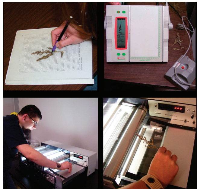
Figure 1. Dot grid (top left), ADC AM300 portable scanner (top right; ADC BioScientific Ltd., Hoddesdon, England), and LI-COR LI-3000 desktop scanner (bottom; LI-COR Inc., Lincoln, NE) used to estimate seed-head area for predicting seed production of moist-soil plants, Tennessee National Wildlife Refuge, USA, September 2005 and 2006.
