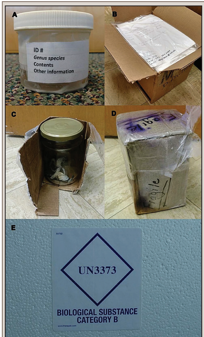
FIG. 4. Examples of packaging samples for shipment. Photos A and B show proper packaging using plastic containers with screw top lids and shipping within a styrofoam cooler in a tertiary cardboard box. Contents of the package are included in a packing slip. Absorbent material (paper towel) and cushioning have been added. Photos C and D show types of packaging that should be avoided. Glass jars with lightly twisted lids can easily break or leak in shipment. All shipments should have three layers of packaging with absorbent material to handle any leakage and provide cushioning. Contents should be labeled as per the requirements of the commercial carrier and at minimum labeled as diagnostic specimens. A packing slip with a list of all samples included in the shipment should be included and it is best to place it in a sealable plastic bag in case of any leakage. Photo E shows an appropriate biohazard label for a Category B biological specimen, which includes all diagnostic specimens.
